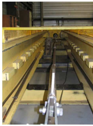
Tensile test up to 70 T
