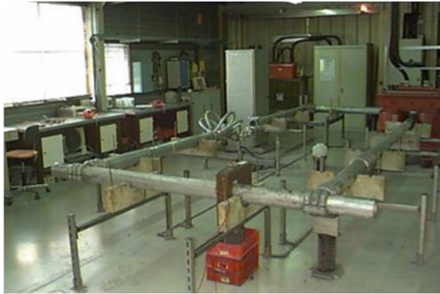
Temperature rise test up to 10kA
