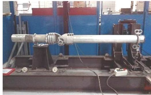
Cantilever/Bending test up to 5T/Axis
